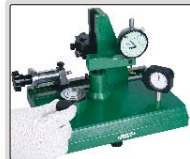
Test force of dial indicators
